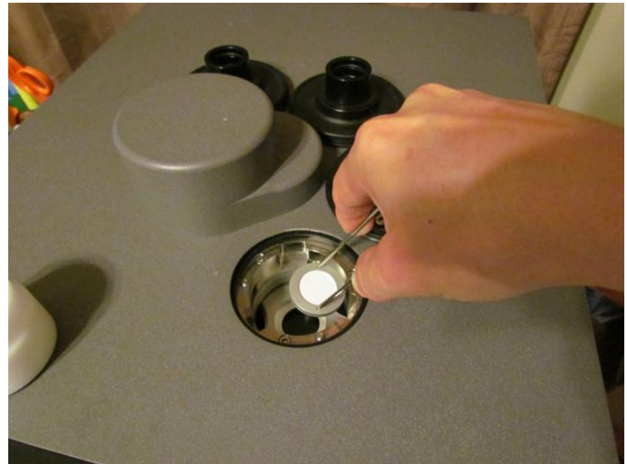
Fig 1. Inserting spy filter into position
